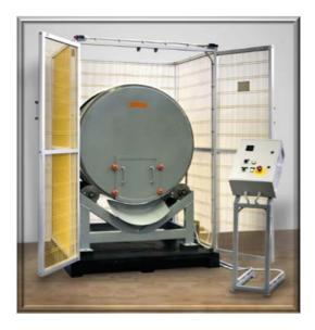
Tumbler Systems to mechanically test samples of coke, coal, iron ore, iron ore pellets according to several international standards.
